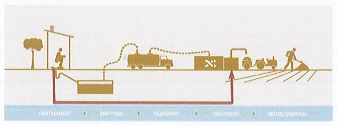
Here toilet construction technologies will ensure safe containment of other on-site systems human faeces from the will be undertaken in environment
